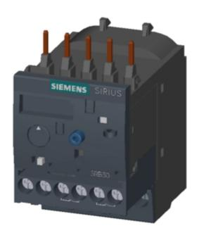
Overload relay 4...16 A for motor protection Size S00, Class 20E Contactor mounting Main circuit: Screw Auxiliary circuit: Screw Manual-Automatic-Reset
