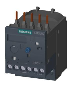
Overload relay 0.32...1.25 A for motor protection Size S00, Class 20E Contactor mounting Main circuit: Screw Auxiliary circuit: Screw Manual-Automatic-Reset
