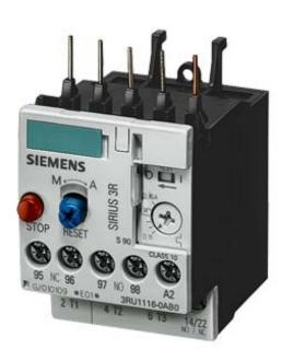
Overload relay 0.11...0.16 A For motor protection Size S00, Class 10 Contactor mounting Main circuit: screw terminal Auxiliary circuit: screw terminal Manual-Automatic-Reset !!! Phased-out product !!! Successor is SIRIUS 3RU2 Preferred successor type is >>3RU2116-0AB0<<
