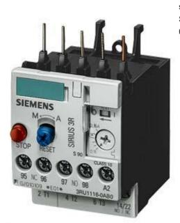
Overload relay 0.7...1 A For motor protection Size S00, Class 10 Contactor mounting Main circuit: screw terminal Auxiliary circuit: screw terminal Manual-Automatic-Reset !!! Phased-out product !!! Successor is SIRIUS 3RU2 Preferred successor type is >>3RU2116-0JB0<<
