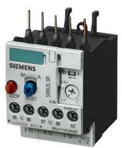
Overload relay 1.4...2 A For motor protection Size S00, Class 10 Contactor mounting Main circuit: screw terminal Auxiliary circuit: screw terminal Manual-Automatic-Reset !!! Phased-out product !!! Successor is SIRIUS 3RU2 Preferred successor type is >>3RU2116-1BB0<<
