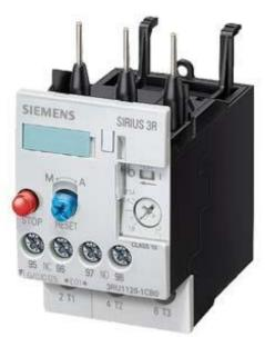
Overload relay 20...25 A For motor protection Size S0, Class 10 Contactor mounting Main circuit: screw terminal Auxiliary circuit: screw terminal Manual-Automatic-Reset !!! Phased-out product !!! Successor is SIRIUS 3RU2 Preferred successor type is >>3RU2126-4DB0<<
